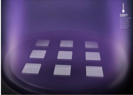
Slices of synthetic diamond are used as the starter “seed” and placed in a high output microwave chamber. Methane and Hydrogen gasses are added, and a plasma field is created.
