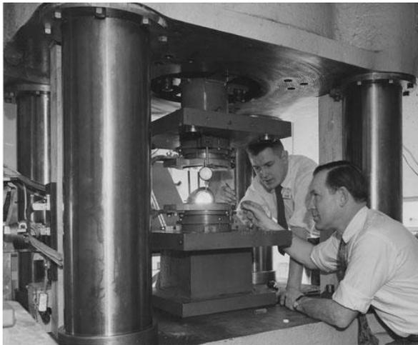
General Electric Scientists using a high pressure press to make the first synthetic diamond in 1955.
