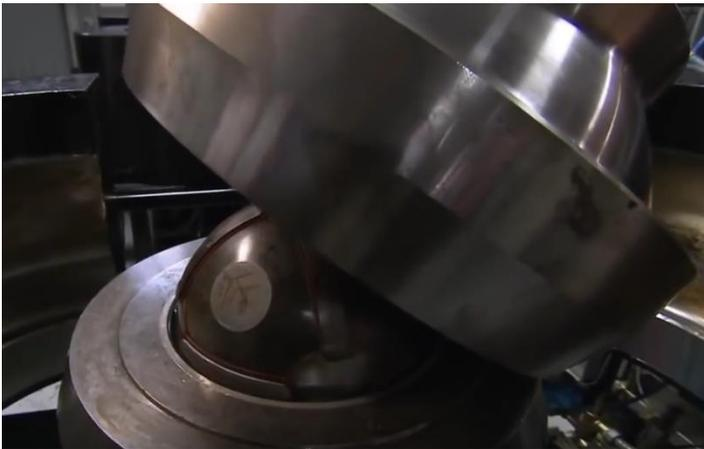
The vessel is placed in a pressure chamber where pressures 50,000 times greater than our atmosphere are created and temperatures exceed 2,300 degrees Fahrenheit.
